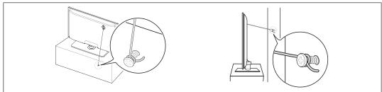
4. Verify all connections are properly secured. Periodically check the connections for any sign of fatigue or failure. If you have any doubt about the security of your connections, contact a professional installer.
